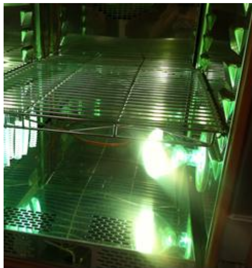
Figure 2: Samples arrangement in the climatic test chamber during the UV-ageing test.
